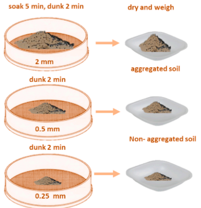
Fig. 2. Wet sieve soil aggregation test. Soil added to the sieve set is soaked and dunked twice per min for 2 min. Soil on top sieve is then dried and weighed. The process is repeated for the next sieves.
