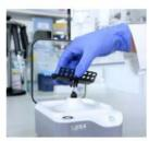
Quick and Easy Rotor Change - To mount one of the two rotors, simply push it onto the drive shaft until there is an audible click. Remove it by pulling it straight up and off the shaft.
