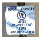
Refrain from: Daisvchaining RPTs (connected together), or use with extension cords.
